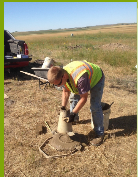
Material Tester Sasha Johnson performing a slump test.
