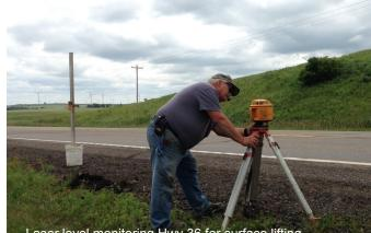
Laser level monitoring Hwy 36 for surface lifting.
