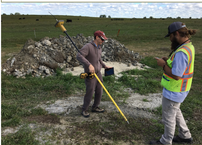
PSC staff are surveying drill holes in the north ditch of Highway 36 between 41 st Street and 52 nd Street.
