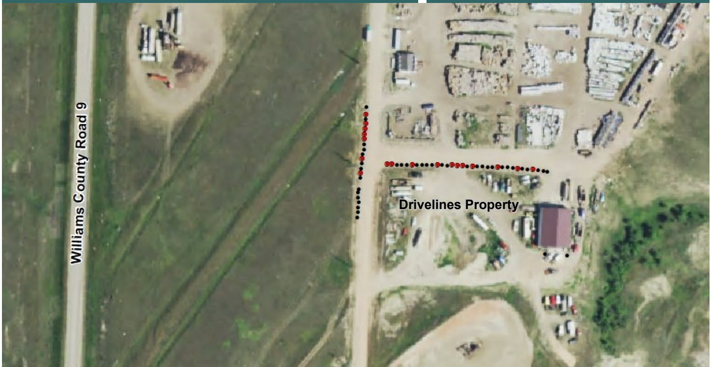
Williams County Road 9 , also called 134 th Avenue NW, runs north and south. Drilling encountered solid coal at black dots and no coal at black triangles . Red dots are void holes that need grout.
