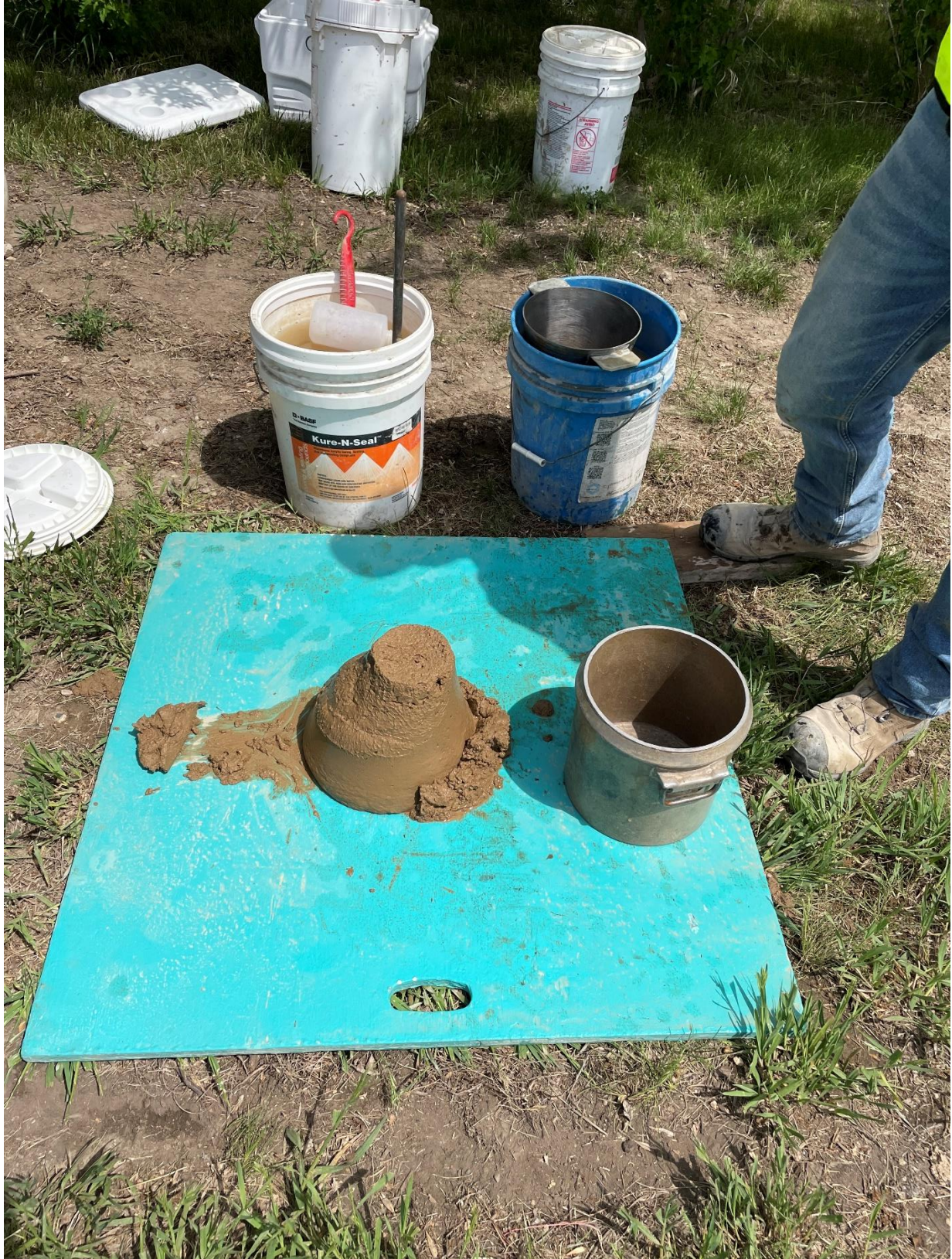
Figure 1: The material testing contractor is performing a grout slump test.
