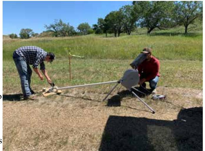
*PSC Staff Using a Borehole Camera to Inspect Underground Mine Workings at Noonan*
