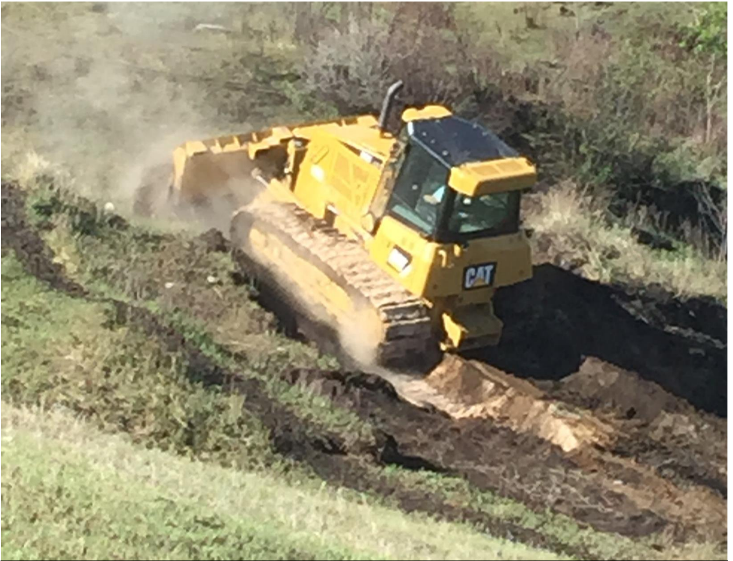
Above: Dozer pushing hot ash into pile for burial, average temperature 500°.
