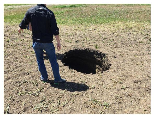
This shows AML employee, Jordan Burns, inspecting a sinkhole on a cropland field near New Salem. Although small in diameter at the surface, beneath the surface this dangerous sinkhole was 12 feet long, five feet wide and five feet deep.
